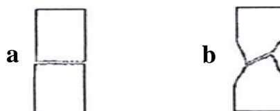
Figure 2. (a) Fracture pattern of brittle material (b) fracture pattern of ductile material.
